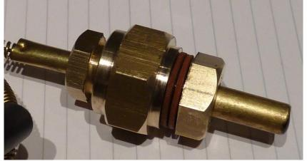
So, then, it was simple task of turning-up an adapter bush (from 1" AF brass hexagon) to accept the sender and include a male threaded spigot to pass through a ½" hole in the tank wall. The bush was secured with a fibre washer either side of the tank
